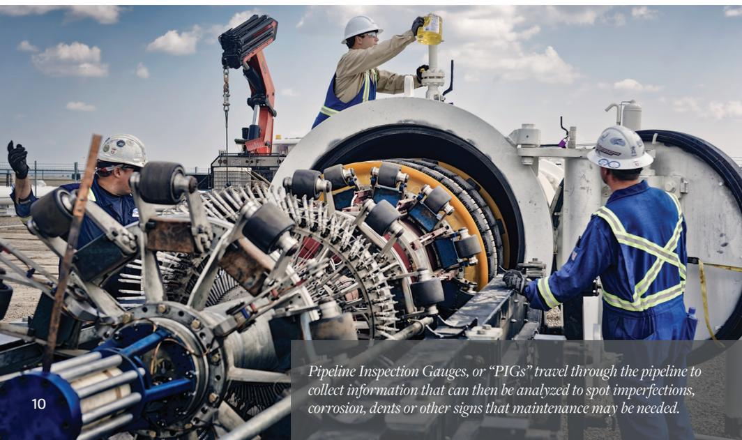
*Pipeline Inspection Gauges, or “PIGs” travel through the pipeline to collect information that can then be analyzed to spot imperfections, corrosion, dents or other signs that maintenance may be needed.*
